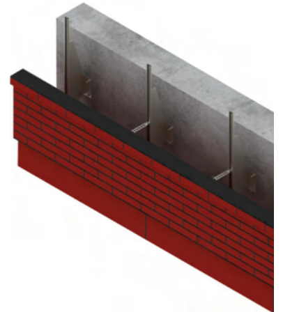
• Brickwork facing walls restraining system with HMS-AV restraint channels & ties
