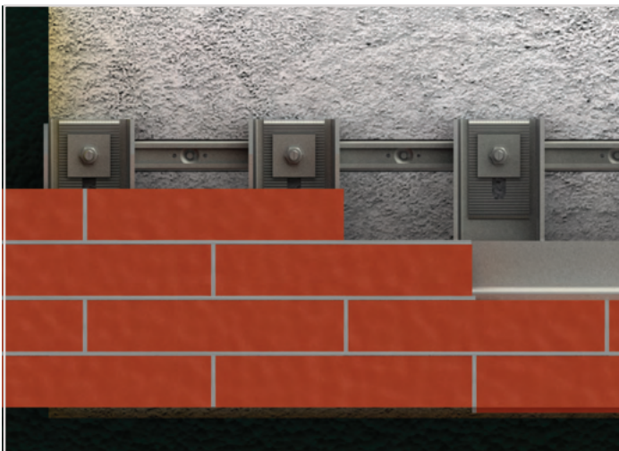
• Elevation picture of brick facing installation with HMCS supports
