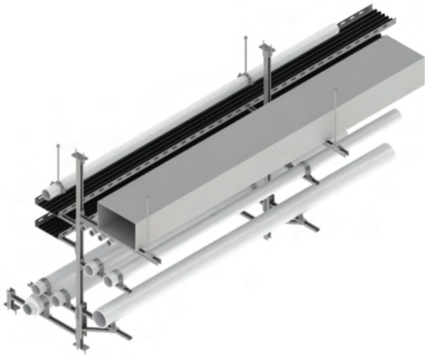
• Installation of pipe and duct systems.
