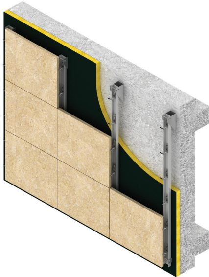
Sub Channel Fixing System with Vertically & Horizontally spanned channels
